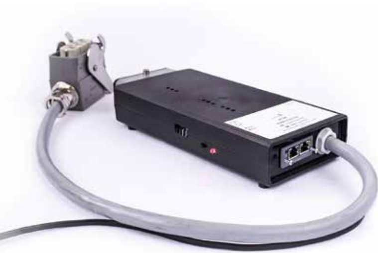
Fig. 3. Power measurement device for DC industrial robot and measurement performance evaluation example against oscilloscope based power measurement
