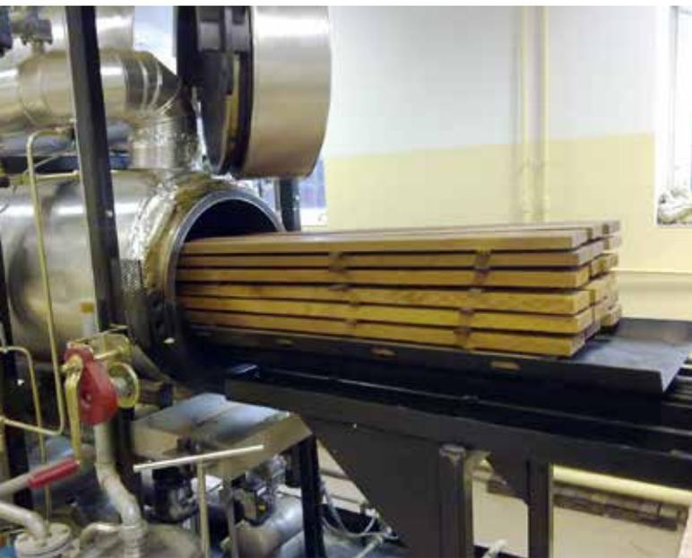
Wood thermally modified in a pilot plant.
