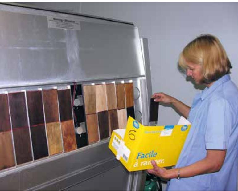
Dr. D. Cīrule prepares a test for artificial aging of wood in a chamber
