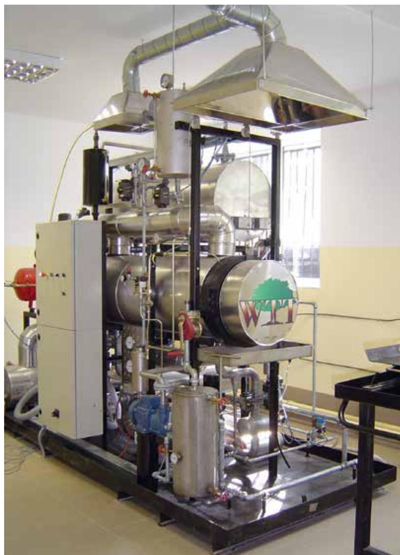
Pilot plant for hydrothermal modification of wood (WTT, Denmark)
